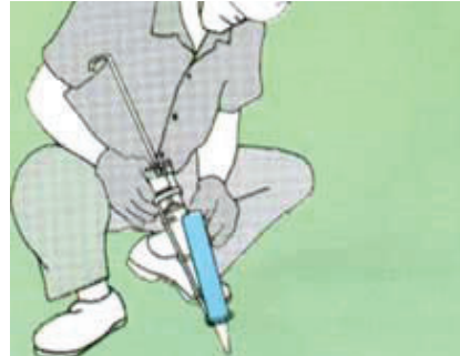
4. Set the cartridge to the caulking gun.
