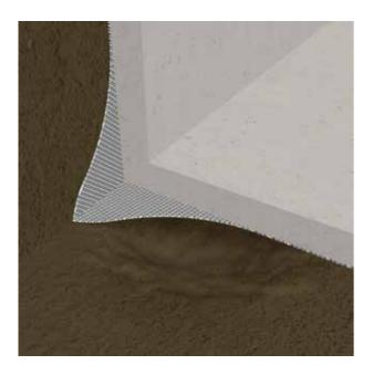
PVC membranes, self-adhesive and torch-on membranes can collapse where ground settlement takes place.
