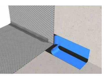
Floor/Wall transitions are easily achieved using Proofex "L" section rolls. The blue release film is peeled off leaving a sticky butyl adhesive on to which the Proofex Engage is attached.
