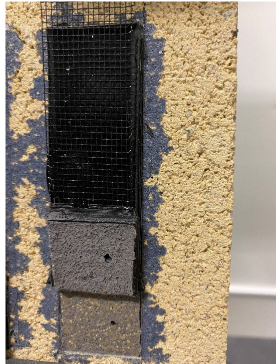
FIGURE 4 IMAGES OF TEST SAMPLE PERFORMING ADHESION-IN-PEEL
