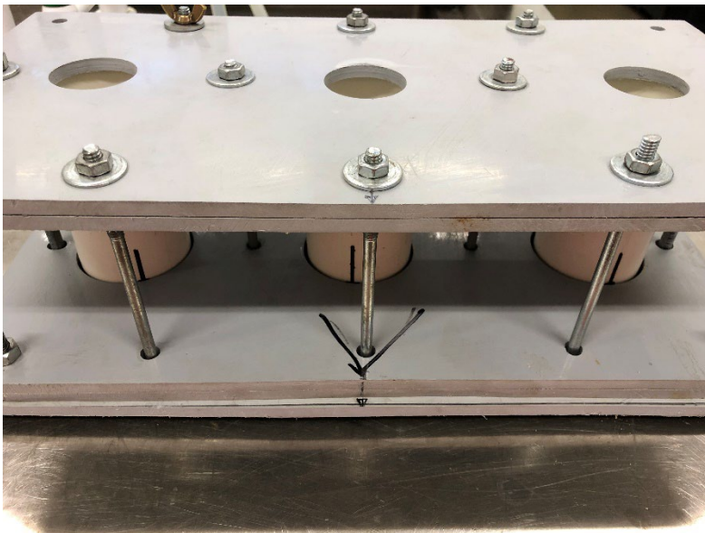
Figure 3 Test apparatus and weighing of Nitoproof 910 - Waterproofing Membrane
