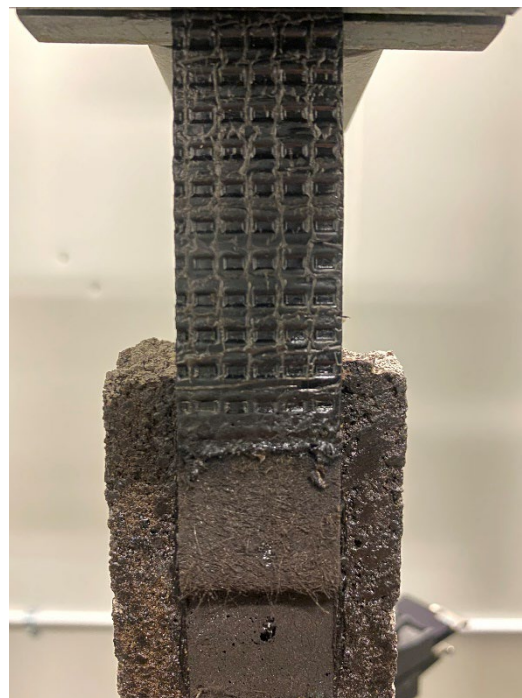
FIGURE 4 IMAGES OF TEST SAMPLE PERFORMING ADHESION-IN-PEEL
