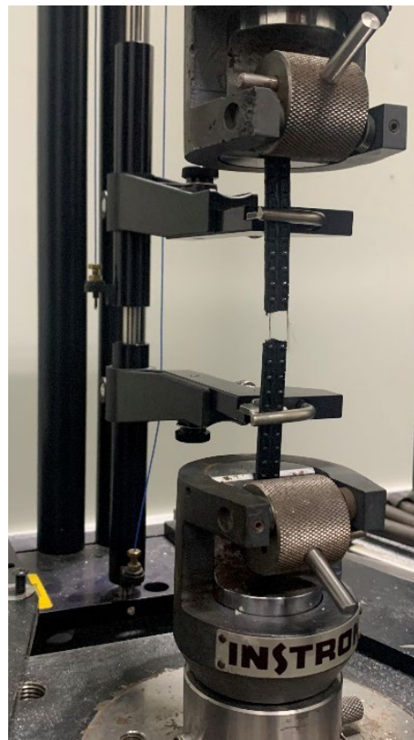
FIGURE 3 IMAGES OF TEST SAMPLE PERFORMING DURABILITY LOAD / ELONGATION TEST
