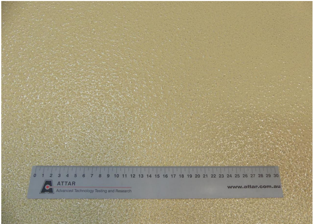
Figure 1: Fosroc Nitoflor FC150 HP + Fosroc Nitoflor Anti-Slip Grains 01 Silica Sand 16/30# + Fosroc Nitoflor PA
