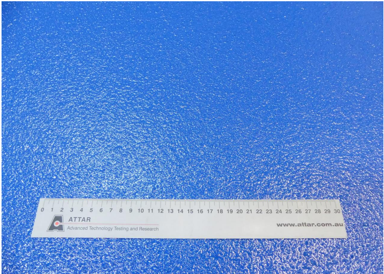
Figure 1: Fosroc Nitoflor PU 600 + Fosroc Nitoflor Anti-Slip Grains 01 Silica Sand 16/30# + Fosroc Nitoflor PA
