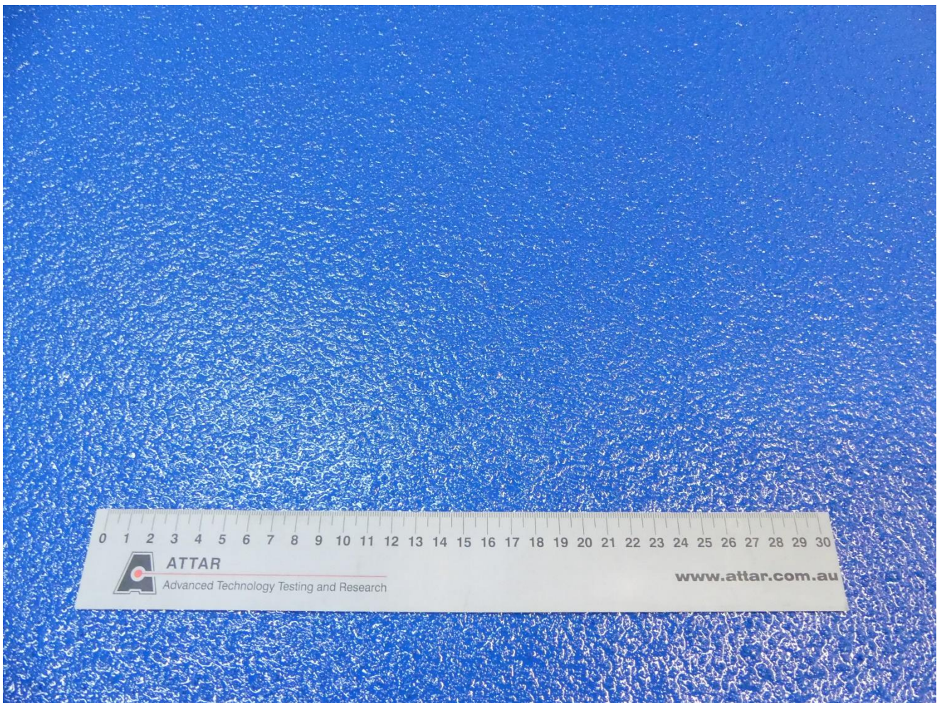
Figure 1: Fosroc Nitoflor PU600 + Fosroc Nitoflor Anti-Slip Grains 01 Silica Sand 16/30# + Fosroc Nitoflor PA.
