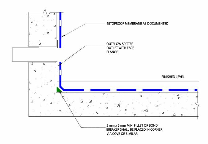
NITOPROOF - OVERFLOW PIPE PRE-FORMED SPITTER THROUGH PARAPET
