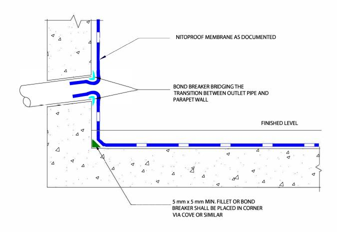
NITOPROOF-OVERFLOW PIPE THROUGH PARAPET DETAIL
