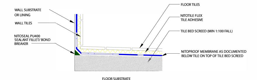
NOTE: WATERPROOF MEMBRANES SHOULD BE TERMINATED AT A MINIMUM HEIGHT OF 150mm ABOVE FINISHED FLOOR LEVEL (EXCEPT IN SHOWER AREAS)
