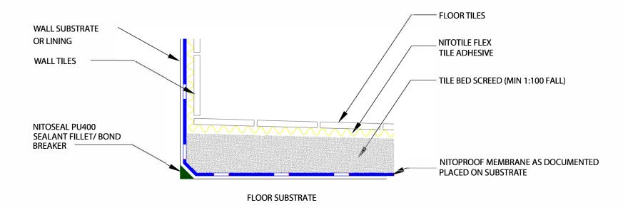
NOTE: WATERPROOF MEMBRANES SHOULD BE TERMINATED AT A MINIMUM HEIGHT OF 150mm ABOVE FINISHED FLOOR LEVEL (EXCEPT IN SHOWER AREAS). WATERPROOF ENTIRE FLOOR AREA.
