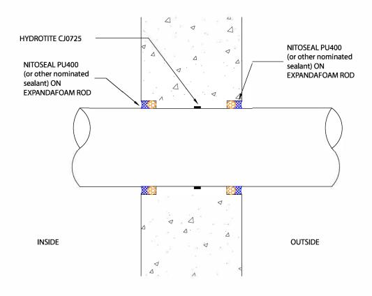
NITOSEAL/HYDROTITE - PIPE THROUGH WALL DETAIL
