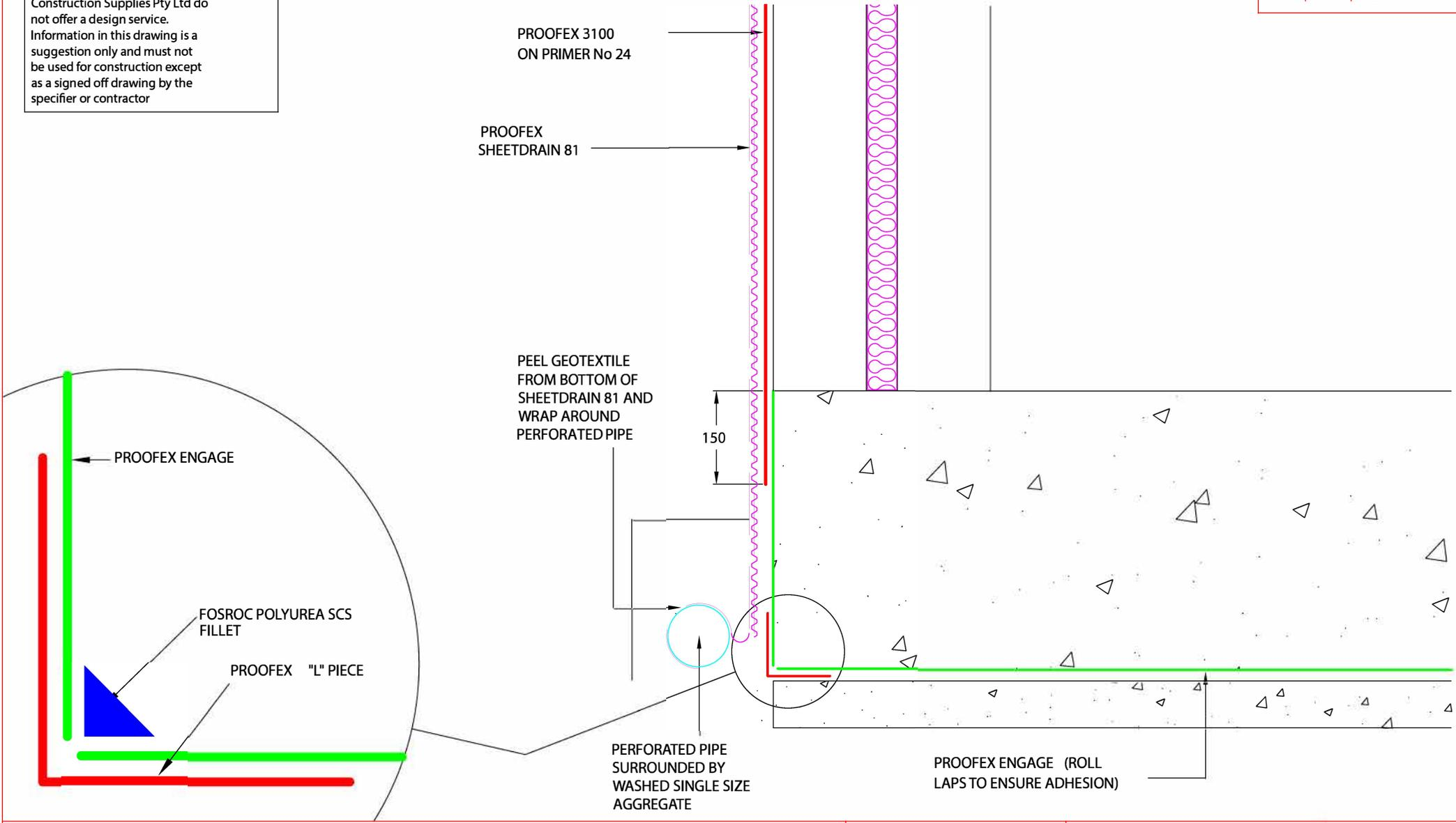
**PROOFEX ENGAGE - BASEMENT BLOCKWORK WALL/SLAB CORNER DETAIL**
