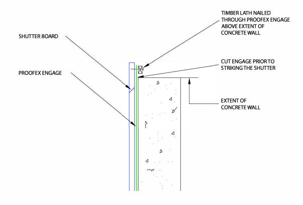
PROOFEX ENGAGE - FIXING DETAIL ABOVE EXTENT OF CONCRETE WALL
