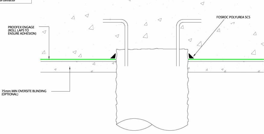
PROOFEX ENGAGE - PILE HEAD DETAIL (a)
