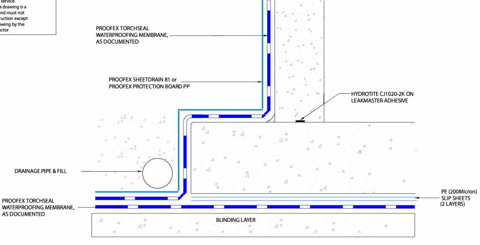
PROOFEX TORCHSEAL - BASEMENT SLAB TO WALL EDGE DETAIL
