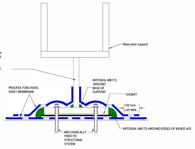
PROOFEX TORCHSEAL - DETAILING OF METAL POST SUPPORT - AFTER MEMBRANE INSTALLATION
