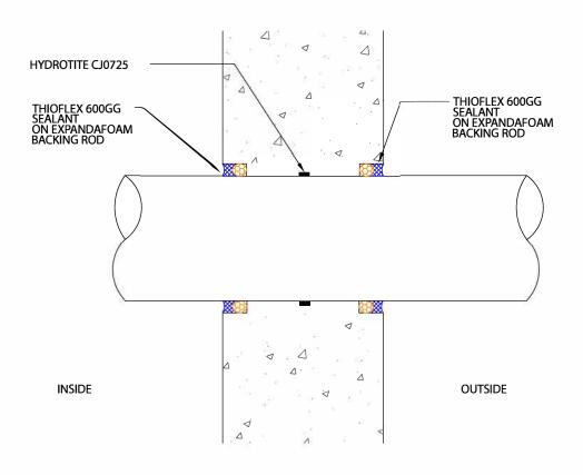
THIOFLEX 600GG / HYDROTITE - FUEL PIPE THROUGH WALL DETAIL
