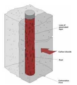
CO2 is a naturally occurring gas and enters every concrete, especially in mid-range humidity. The slightly acidic nature of the Carbon Dioxide, weakens the protective alkaline nature of the concrete and slowly permeates to the level of the steel. Once at the steel, it changes the naturally protective environment into one that is neutral and erodes the passivating film on the steel. In this environment the presence of moisture and oxygen begin the corrosion process.
