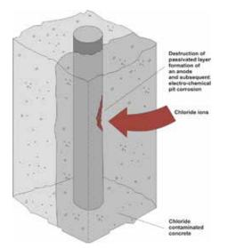
Chlorides can enter concrete for a variety of different reasons, the most common are from a marine environment or use of de-icing salts. Chlorides may also be bound into the concrete during its initial casting, by use of accelerators or unwashed sands and aggregates.
